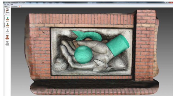
Figure 2: Supported Areas in the 3D annotation process; a Sphere for the loaf, a Cylinder for the arm and a Segment for the fish tail
