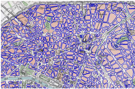
Figure 10: A set of building footprints (shown in blue) extracted from a map of Paris from 1879. The automatic process returned 1123 valid building shapes for the whole map. The results shown here are before any manual editing has taken place.
