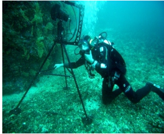
Figure 3. The acoustic camera in situ, just in front of the cave (see next image).
