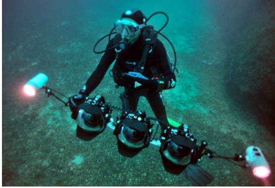
Figure 5. The photogrammetric survey with the Menci approach (Three synchronized digital camera).
