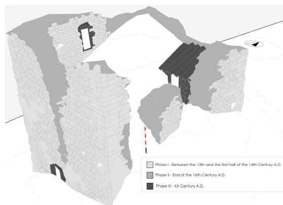
Figure 5: Three-dimensional survey of wall stratigraphy with identification of different building phases.
