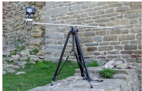
Figure 4: The photographic tripod used to perform stereo-pairs.
