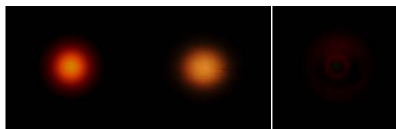
Figure 4: Left, simulated subsurface scattering penetrating the virtual marble sample. Centre: photograph of light penetrating the marble sample. Right: The difference between the two images.
