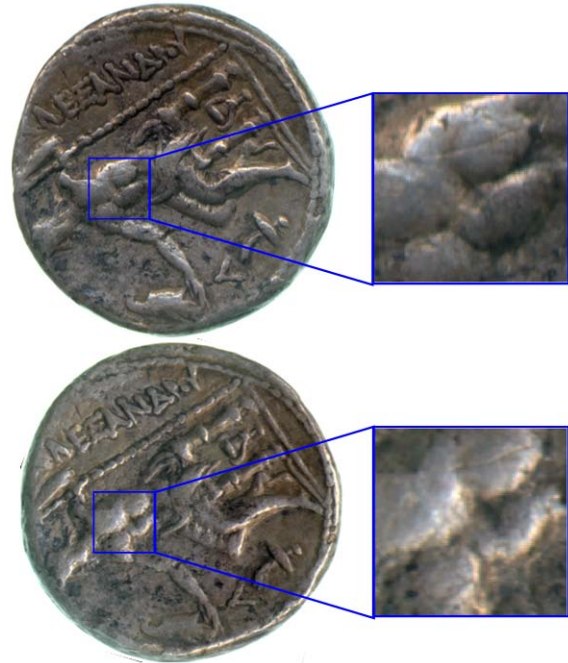
Figure 3: Two images of the same coin, illuminated from different directions. A high variation of specular reflections can be seen due to the surface characteristics of the coin.
