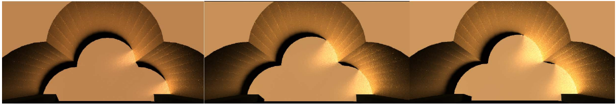
Figure 9: Schematic evolution of the back lighting of the heads kings due to caustics formation by reflection of the solar light at sunset. Light is guided by a grazing and progressive reflection on the gilded cylindrical shapes of the arcatures. From left to right the solar spectrum slightly changes according to the spectrophometric emission measurements made from 21:09 to 21:33 on 2009 July 15th.
