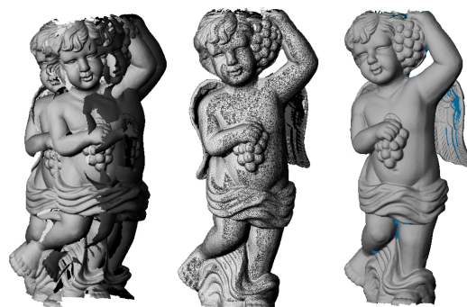
Figure 6: Process from single scans to merged polygonal mesh.
