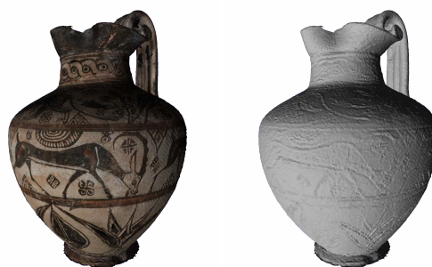
Figure 9: The rendered surface on the right shows some geometric aliasing due to improper acquisition on the discontinuity border of painted regions, visible on the leftmost image.
