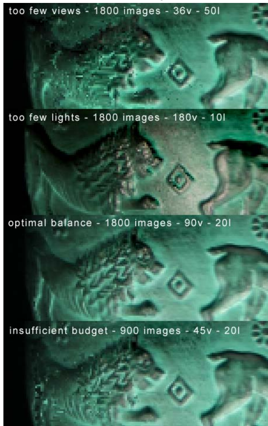
Figure 9: Interpolating between too few views results in artifacts, as does interpolating between too few lights. Choosing the optimal tradeoff between lights and views results in interpolation with no visible errors. If the image budget is too small, even the optimal tradeoff will contain noticeable artifacts.
