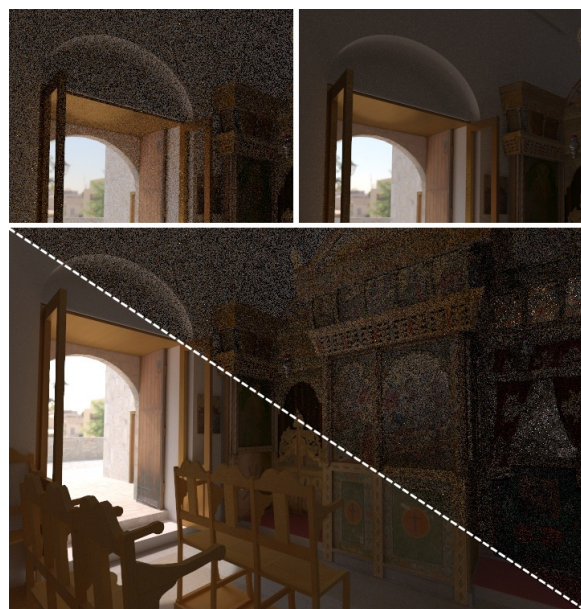
Figure 9: Top: Comparison of the doorway. Bottom: Two Path Traced images combined into one. Top half: 200 samples per pixel. Bottom half: 16,000 samples per pixel.
