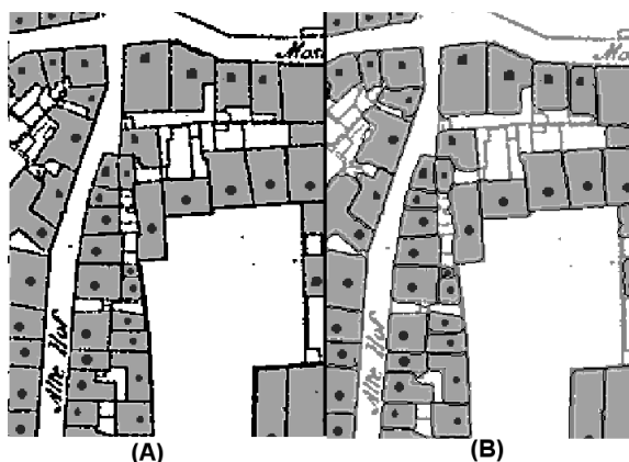
Figure 4: (A) From each black building indicator point a seed fill algorithm is performed to construct the dark grey building areas. The initial building footprint polygons are shown in light grey surrounding each building area. (B) By employing an active contour model the footprints are adjusted to fit to the centres of the building footprint edges in the map.
