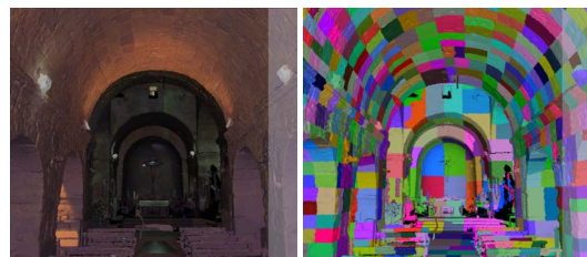
Figure 4: Sant'Antioco Basilica. Patch refinement: 1665 patches with a total of 1.3M samples, rendered at 100 fps on a 1024x768 window, with elliptical splats enabled.
