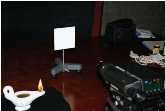
Figure 10: The light emitted by the lamp (left) is almost entirely reflected in the white board (middle) which is then captured by the spectroradiometer (right).
