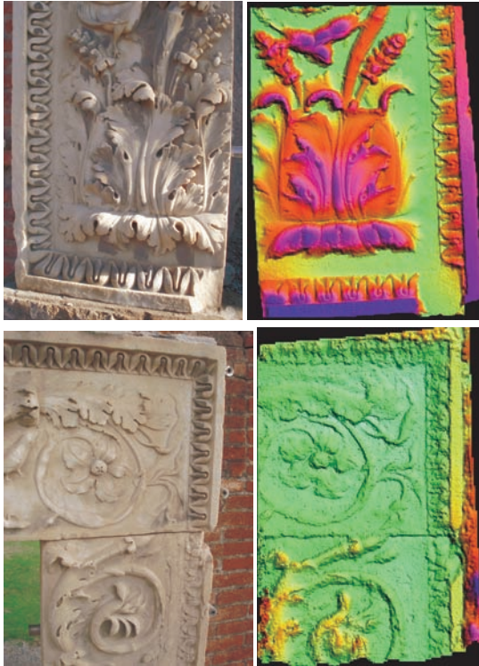
Figure 5: Detailed ornaments modeled by means of dense image matching and derived surface models shown in colour-code mode.
