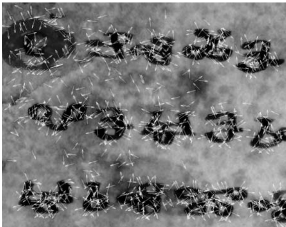
Figure 3: Detail of a test image. The white arrows illustrate the orientation for each control point. Since the scale-space is not computed, all control points have the same scale.
