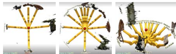
Figure 6: Presentation layout: Chandelier. Even when densely populated, the selected object sticks out clearly due to the uneven circular spacing.
