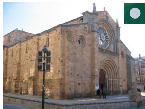
Figure 4: Original image with special targets (3008x2000 pixels)
