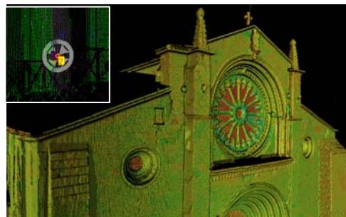
Figure 6: Laser model and the special targets extracted.
