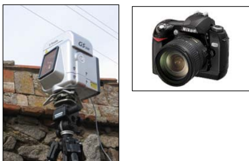
Figure 1: Trimble GS200 laser scanner and digital camera, Nikon D70.
