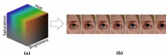
Figure 8: The HSB space is constrained to a three dimensional color space with the following parameters (a): hue from 20 to 250, saturation from 30 to 80 and brightness from 40 to 100. Colors are then randomly chosen inside this space to add variety on the eyes texture of a character (b).
