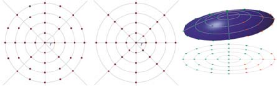
Figure 2: Descriptor layout. Left: The number of sample points per ring grows linear with respect to its length, i.e. the sampling rate for each ring is identical (Four samples per 2\pi r in the depicted case). Centre: Descriptor as suggested in [ZG04]; here, the number of sample points per ring is constant, such that the sampling rate decreases linearly. Right: 3D illustration of the local resampling.
