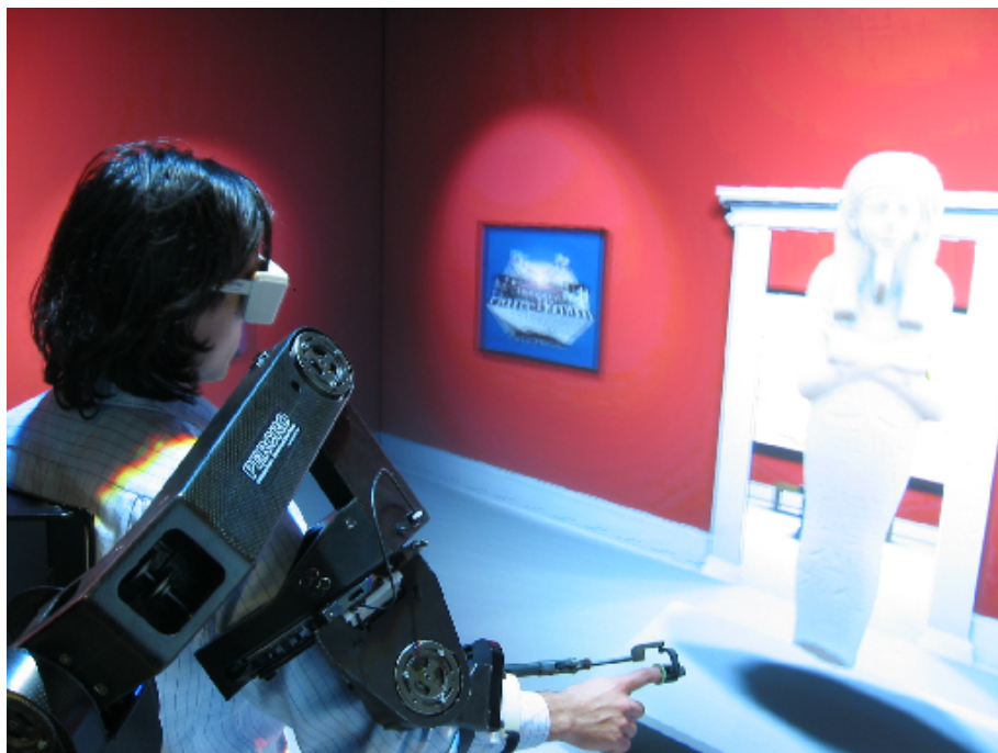
Figure 1: The Museum of Pure Form tested in the ReaCToR. The user touches the statue via a two-point-contact haptic device mounted on an exoskeleton.
