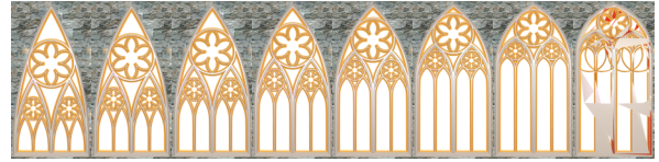
Figure 19: Varying excess with constant height. With a style library, a manifold of windows is obtained using just a few high-level parameters. The mesh is robust against invalid parameters (last image), the parameter validity should be checked on a higher software layer.
