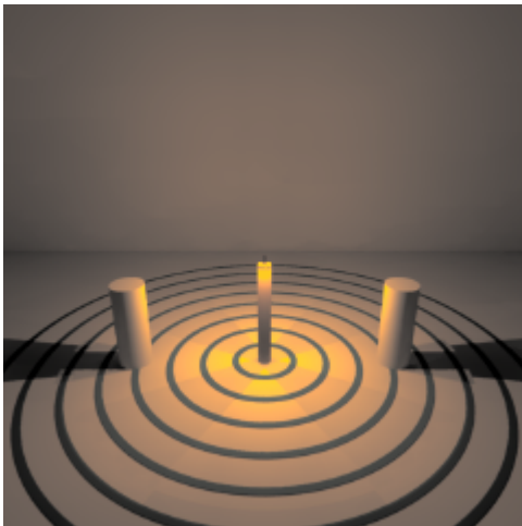
Figure 6: Bounding volume cube as flame light source, artifacts are more than obvious
