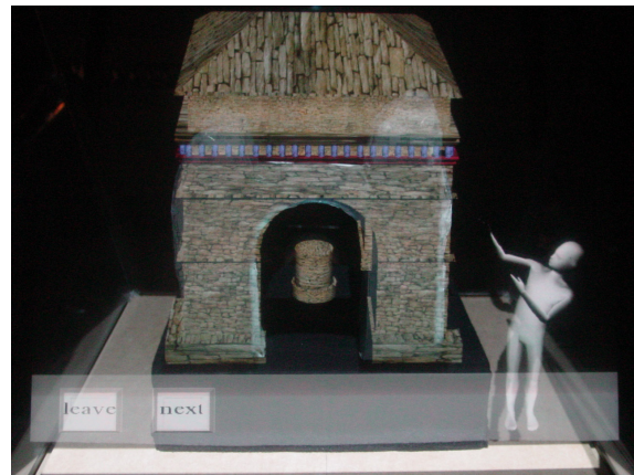
Figure 3: An animated virtual character introduces the Heidentor. Here, the real model remains dark, and is fully replaced by a stereoscopic image of the reconstruction.
