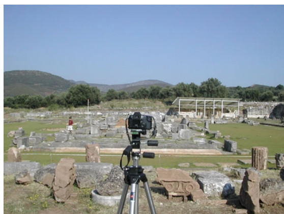
Figure 4: Hundreds of images from at least four different points of view were taken and calibrated in order to create a photorealistic 3D virtual environment of the site.
