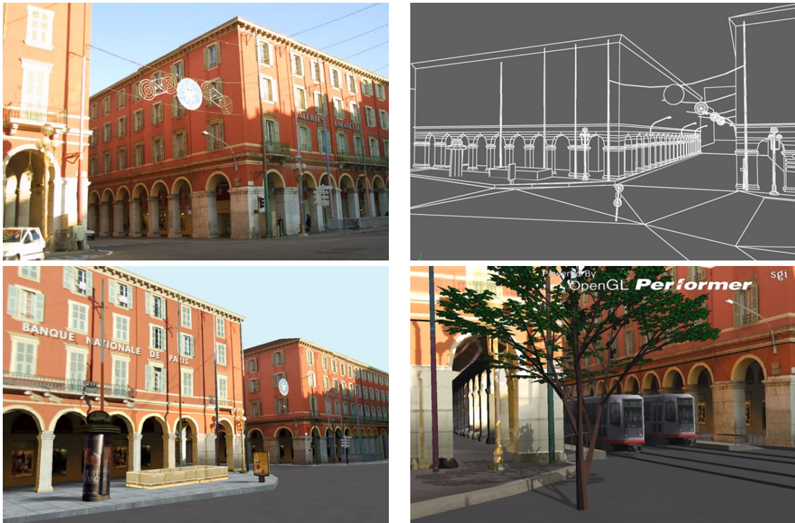
Figure 3: Upper row, left: A photograph of the historical buildings of Place Massena in Nice. Right: Wireframe of the 3D model reconstructed from a series of such images. Lower left, a virtual image of a textured version of the above model. Lower right, addition of virtual elements, realistic shadows and lighting.
