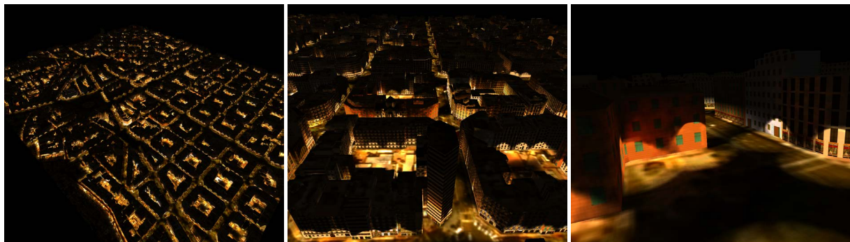
Figure 1: Our algorithm computes an initial approximate solution for the illumination of a city (suitable for far views) which is then refined locally on-demand using photon mapping.
