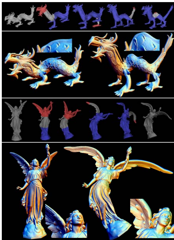
Figure 9: Top: XYZRGB Dragon (7M triangles, interactively deformed with 160k samples). Bottom: Lucy (28M polygons, 300k samples). Each full session with adaptive simplification, interactive editing and streaming deformation took less than 5 minutes.
