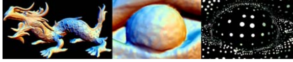
Figure 3: Left: XYZRGB Dragon (7.2M triangles). Middle: Close-up of the eyeball on the original geometry. Right: Adaptive downsampling by out-of-core VS-Tree clustering.
