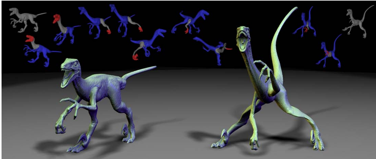
Figure 1: Interactive freeform deformation of the Raptor model (8M triangles). The initial geometry (left) is adaptively down-sampled through a streaming process, to get a simplified point-based version (146k points) that can be edited interactively with on-demand local refinement (blue snapshots). Afterwards, a second streaming process performs a feature preserving deformation reconstruction to the original geometry (right).
