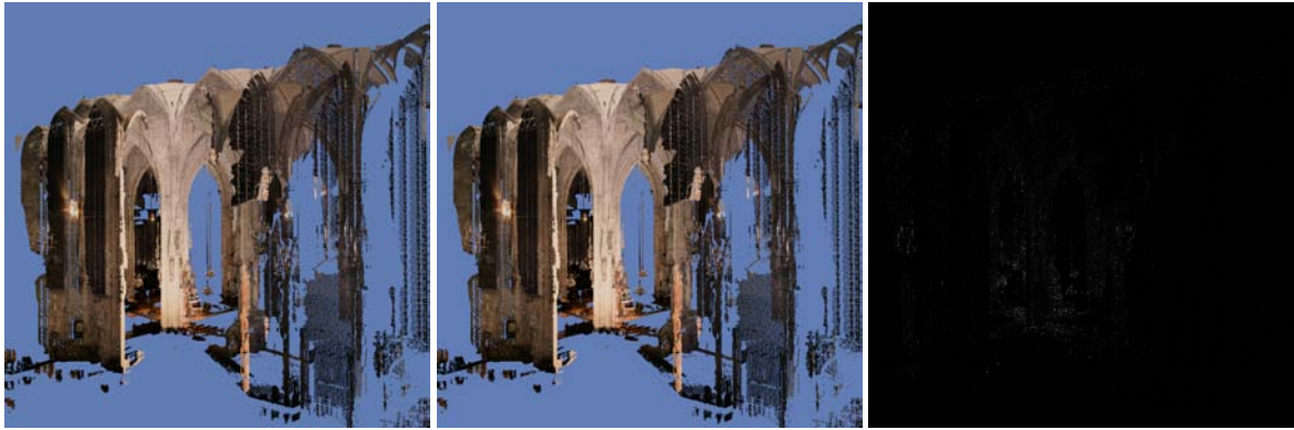
Figure 8: Quality comparison of SPT (left) and MOSPT (middle) rendering. The colors for the SPT were obtained by averaging, those in MOSPT come from selecting representative colors from child nodes. While the difference image (right) does show some discrepancies, the order of magnitude of these differences is not higher than that of the noise contained in the original data.
