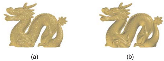
Figure 8: (a) A noisy mesh-model of a dragon, and (b) the corresponding model whose surface normals were recomputed using our kNN algorithm. The algorithm took about 118 seconds and used 8 neighbors.
