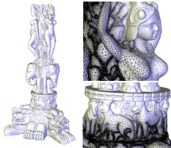
Figure 9: Reconstruction of the THAI STATUE model (5M points) with \rho_{geom} = 0.65 (89% of points removed).
