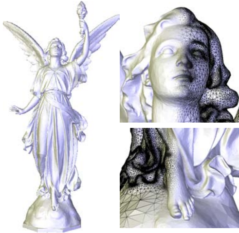
Figure 10: Reconstruction of the LUCY model (14M points), with \rho_{geom} = 0.85 (96% of points removed).
