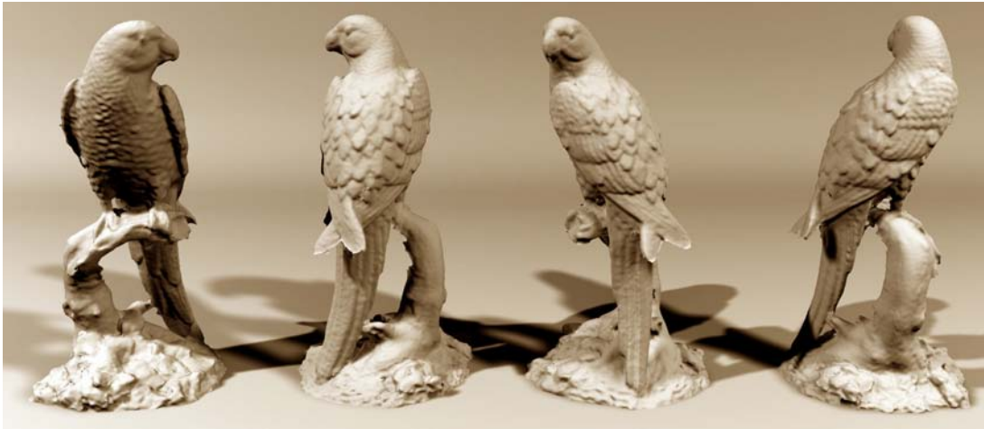
Figure 9: Six super-resolved scans, merged to form a complete model. The original scan data (Figure 2, left) was quite noisy. The super-resolved scans include scanner artifacts, particularly curling at the edges, which had to be trimmed interactively before merging.
