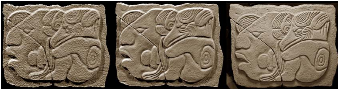
Figure 10: On the left, a single scan of a cast of a Mayan hieroglyphic, with a sample spacing of about 1mm. Center, 90 scans are combined to make a super-resolution surface. Notice the improvement on the eyes, the cross-hatching, and the area in front of the bird's face. Right, a photograph of the cast.
