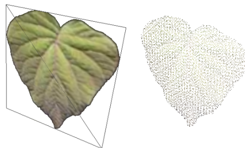
Figure 12: This figure illustrates another benefit of hardware-based sampling. Textured polygons (left) can be sampled according to an alpha-texture and samples are only created only at opaque surface points automatically.
