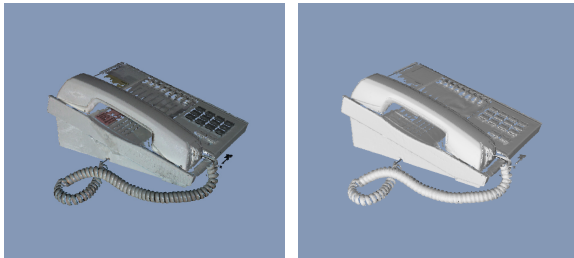
Figure 11: Telephone reconstructed from 15 rotary views (317681 surfels). Lambertian texture (left) and no texture (right).
