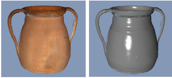
Figure 10: Clay pot reconstructed from 15 rotary views (384492 surfels). Lambertian texture (left) and synthetic Phong texture (right) for showing geometric detail. The Lambertian texture exhibits stripe artifacts due to specular reflection of the clay surface.
