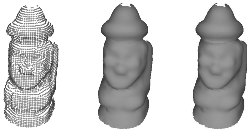
(a) Original cloud (6052 points) (b) Upsampling with MLS (c) Upsampling with ERKPA
