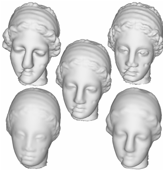
Figure 4: Smoothing and enhancement results of Venus head model. Middle: the original model. Bottom: smoothing. Top: enhancement. Left: large scale. Right: small scale.
