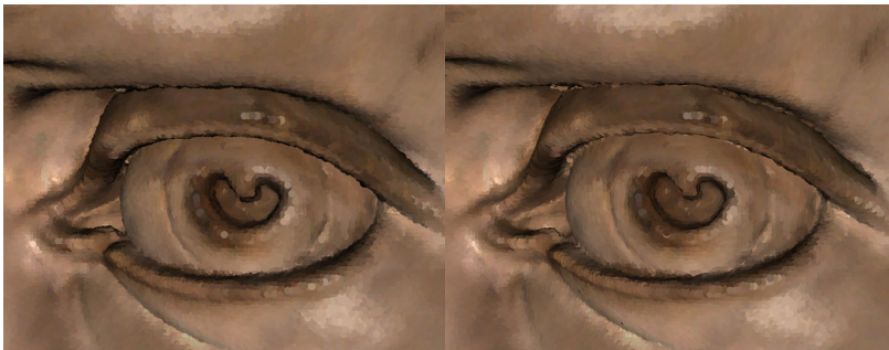
Figure 8: Comparison of rendering quality in QSplat using OpenGL points and oriented disks (left to right).
