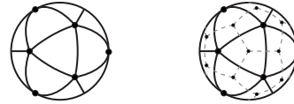
Figure 6: Left: Spherical triangles defined by an icosahedron. Right: The same spherical triangles with the spherical Voronoi diagram illustrated.
