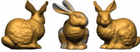
Figure 4: Reconstruction Quality . Reconstruction from 300 simulated noisy scans (point clouds) of the Stanford bunny. In the center, we overlap the reconstructed model with the original model to show error due to dynamic registration. No global error distribution, or data smoothing was performed.
