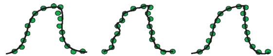
Figure 3: Surface reconstruction from a discrete set of points is an ill-posed problem. The figure demonstrates three possible reconstruction procedures. One which smooths the data, one interpolating the data, and one which allows sharp features.
