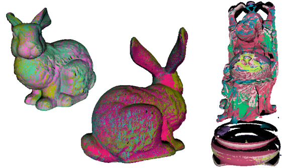
Figure 8: Result of automatic multiview matching and alignment of scans of the bunny and buddha models.
