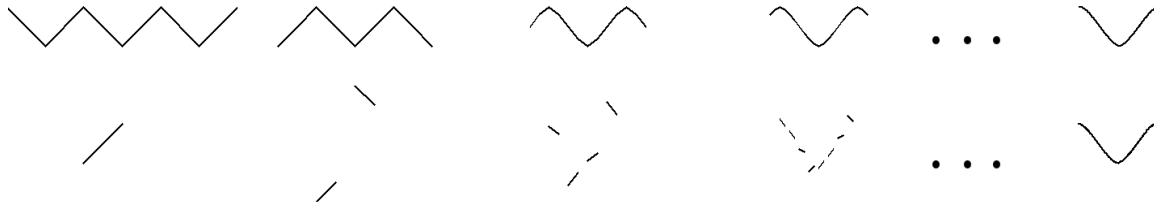
Figure 5: Subdivision using the four-point rule (Top). Starting with a line and iterating the IFS also converges to the same curve (Bottom).
