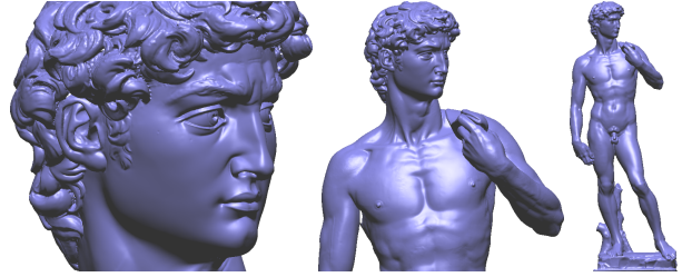
Figure 10: LOD shading of SLIM-approximated David statue. Left: 730 × 650 pixels, 1.7 sec. Middle: 590 × 650 pixels, 1.0 sec. Right: 250 × 650 pixels, 0.4 sec. The image heights are equal and about 650 pixels. Computations were performed on a 3.0 GHz Pentium 4 CPU.
