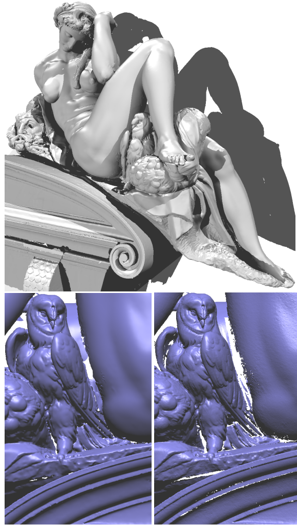
Figure 18: Top: standard ray-traced rendering of a quadratic SLIM-based approximation of the "Night" model with two light sources; original 11 M points are approximated by 432 K quadratic patches; it took 86 sec. for generating the image ( 1000 \times 1000 pixels). Bottom-left: a zoomed fragment of the model approximated and rendered using quadratic SLIM patches. Bottom-right: the same fragment is rendered with our implementation of the Stanford QSplat Multiresolution Point Rendering System (we use our implementation instead of the original one proposed in [RL00] and available online in order to equalize shading effects for the bottom images).
