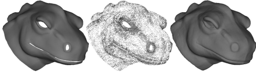
Figure 1: The initial model (left), a non-uniform sampling of points from the model (middle), and the reconstructed water-tight, surface obtained using our method (right).
