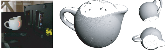
Figure 2: Left: Acquisition setup with Cyberware Desktop 3D Scanner 15 and physical model, right: Raw point cloud obtained from six range images in a single rotational scan. The spiky outliers are artifacts caused by specular reflections.
