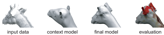
Figure 13: Evaluating the final completed shape. The color-coding in the right image shows the shape matching penalty, where red color indicates insufficient surface completion due to invalid correspondence between input data and context models.
