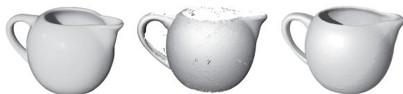
Figure 11: Reconstructed coffee creamer, from left to right: Physical model, acquired data set, reconstructed model.
