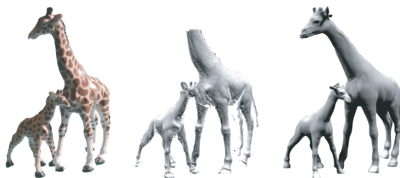
Figure 12: Shape reconstruction from low-quality data, from left to right: Physical model, acquired data set, reconstructed model.
