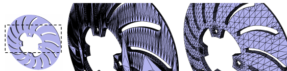
Figure 7: This figure shows the remeshing of a Brake Hub model. The center and right images show the triangulation of the original model and the remeshed model. The original brake hub model has 14K triangles. Our algorithm took 1.85 secs to perform remeshing and generate a mesh with 7K triangles at a Hausdorff error of 1/32 .
