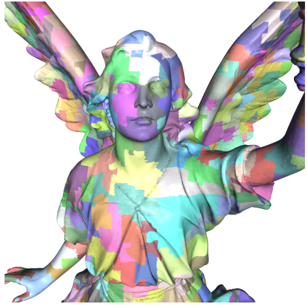
Figure 3: Cluster Decomposition. This figure highlights the clusters on the Lucy model (28M triangles). The average cluster size is 1K triangles. Each cluster is represented by a progressive mesh for dynamic simplification and contains a bounding volume for collision culling.
