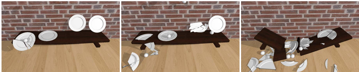
Figure 1: Smashing Plates. The user drops balls in real-time to smash the plates, and at the end of the simulation the scene consists of more than 45K triangles. The complete simulation runs at 8ms per time step on average, with a maximum of 17ms.
