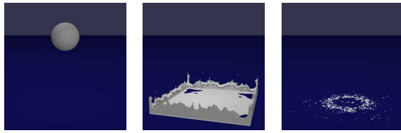
Figure 7: Liquid ball dropped inside a box simulated on a 128^3 resolution grid. Left) Initial condition. Shape of the surface at frame 40 computed with our method (middle) and with PLS (right). PLS loses most of the mass due to the large time step used.
