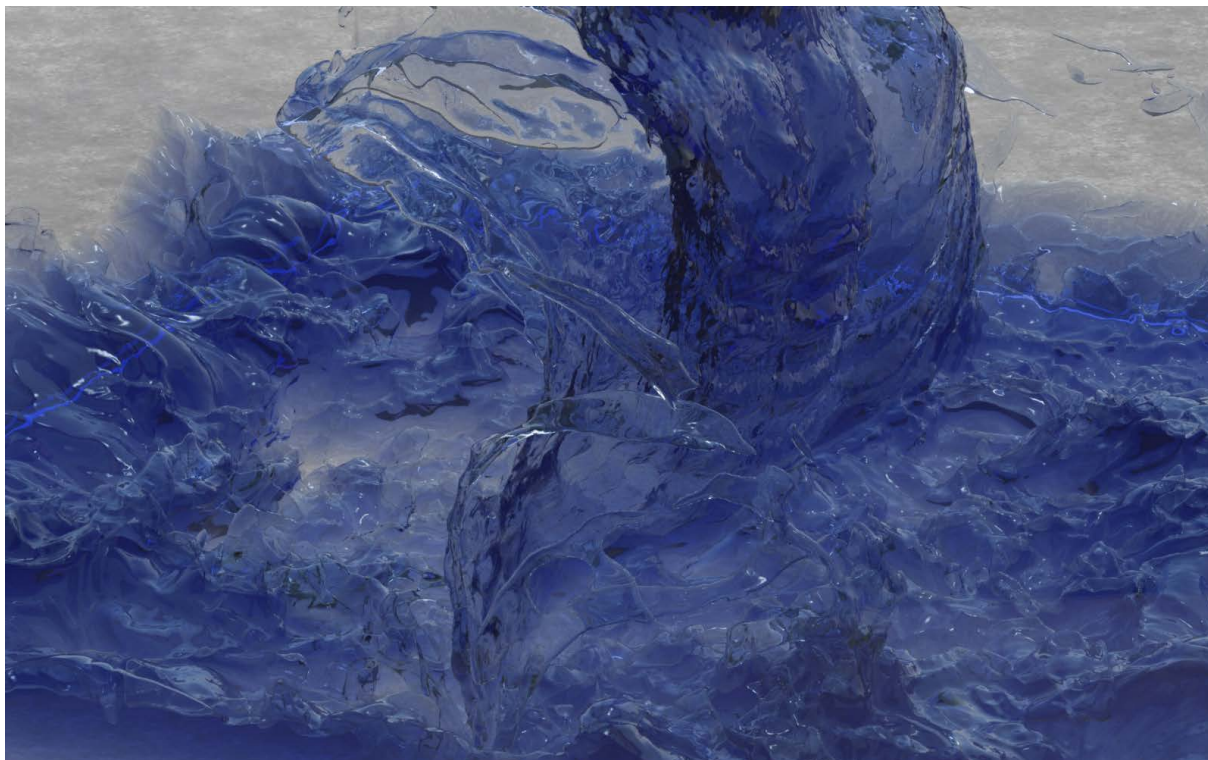
Figure 1: Water pouring into a box at a resolution of 512^3 . This example ran with a CFL number ranging from 10-60 and demonstrates the large amount of small scale details that can be achieved by using our method.
