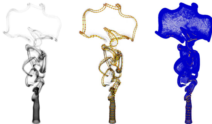
Figure 10: A snapshot of the 1,500th frame of a 30 second, 1,800 frame simulation showing the blurred density ( left ), vortex filaments and smoothed density ( center ), and triangle edges ( right ). The smoke mesh contains 108,711 vertices, and the vorticity graph contains 656 vertices and 694 edges.
