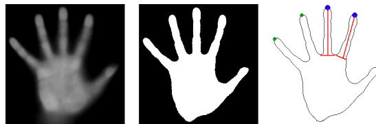
Figure 8: While the Surface can provide approximate depth images (left), appropriate thresholding yields a hand shape (middle) which can be automatically analyzed to identify and measure fingers (right).
